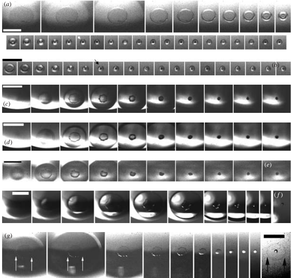
FIGURE 3. Contraction of the air disk, for various impact conditions. (a–e) Water drops D = 4.0 mm. (a) H = 9.7 cm, We = 102 , Re = 6740 , dt = 10 \mu\text{s} . (b) Images from another clip under the same conditions. The arrows point to a trumpet-shaped neck which subsequently pinches off to form a microdrop at the centre, as sketched in figure 8. (c, d) Two realizations for H = 4.4 cm, We = 44 , Re = 4420 , dt = 10 \mu\text{s} . (e) H = 8.2 cm, We = 86 , Re = 6170 , dt = 10 \mu\text{s} . (f) Drop of alcohol, H = 2.5 cm, D = 3.1 mm, We = 50 , Re = 1325 , with dt = 20 \mu\text{s} . (g) More viscous drop, 80% glycerin/water mixture, H = 11.2 cm. We \simeq 160 , Re \simeq 100 . Times shown are 0, 20, 40, 60, 80, 120, 160, 220, 320, 720, 2000 \mu\text{s} . The white arrows point out the location of the edge and the dark arrows point at a faint outer ring of micro-bubbles left behind. The scale bars are 500 \mu\text{m} long.
